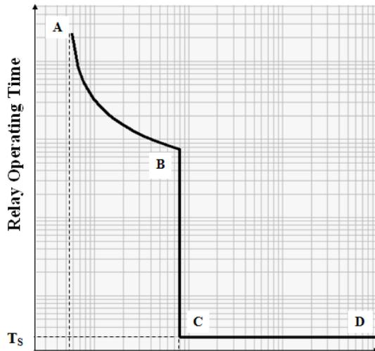
Figure 2: Characteristic curve of OCR [2]
