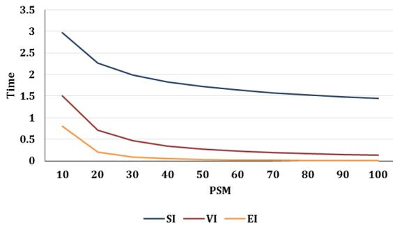
Figure 3: Comparison of SI, VI and EI relays (for TMS = 1.0)
