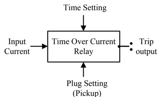
Figure 1: Block Diagram of OCR
