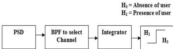
Fig. 3 Representation of energy detector in block diagram.
