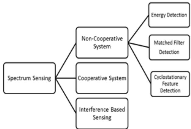
Fig. 2 Classification of Spectrum sensing technique.
