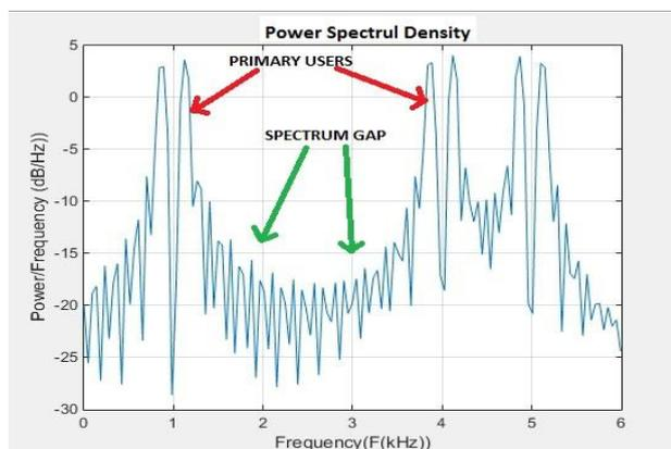
Fig. 5 Used bands (1st, 4th & 5th), and unused bands (2nd & 3rd) graph on MATLAB.
