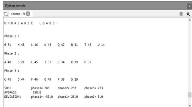
Fig. 5. Before balancing
