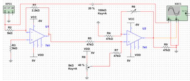
Fig. 3 Signal conditioning simulation circuit
