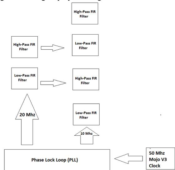
Fig. 5 Block Diagram for the FIR filter operation
