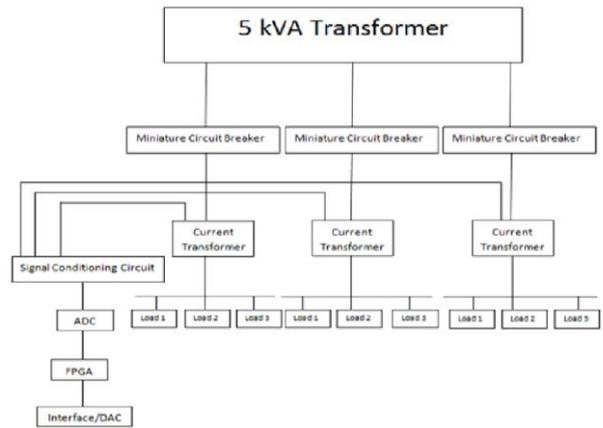
Fig.1 Block diagram of transformer fault analysis test-bench
