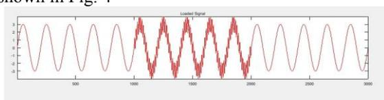
Fig. 4 MATLAB simulation of Highpass filter
