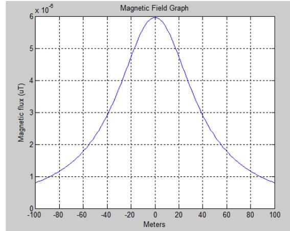
Fig 5: 132 KV Tower Magnetic Field (Rail Conductor)
