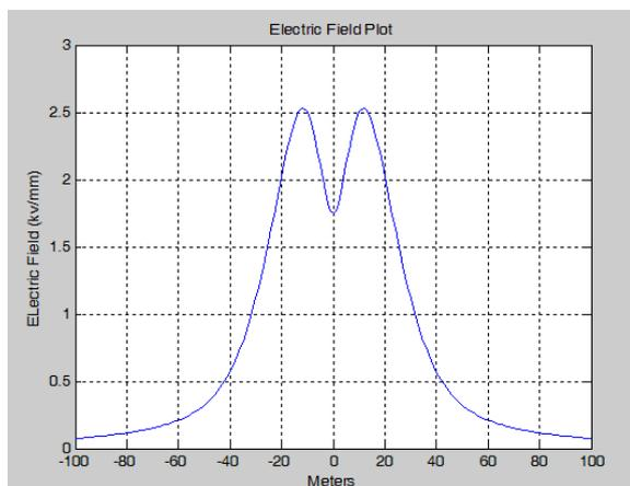
Fig 10: Electric Field Plot 500 KV Tower
