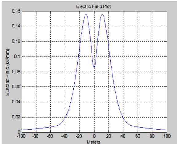
Fig 8: Electric Field Plot 132 KV Tower
