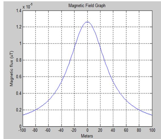
Fig 6: 220 KV Tower Magnetic Field (Curlew Conductor)
