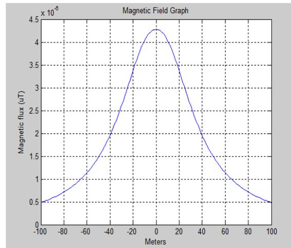
Fig 7: 500 KV Tower Magnetic Field (Merlin Conductor)
