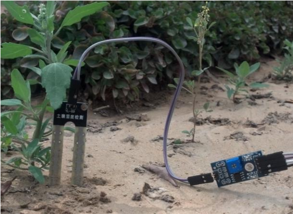
Fig.4: Testing of soil moisture sensor
