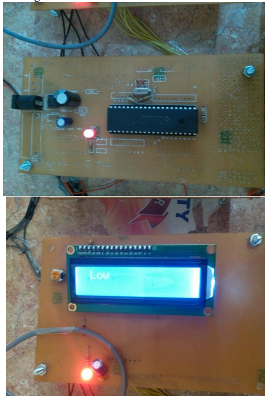
Fig.10 Hardware Board for Level module
